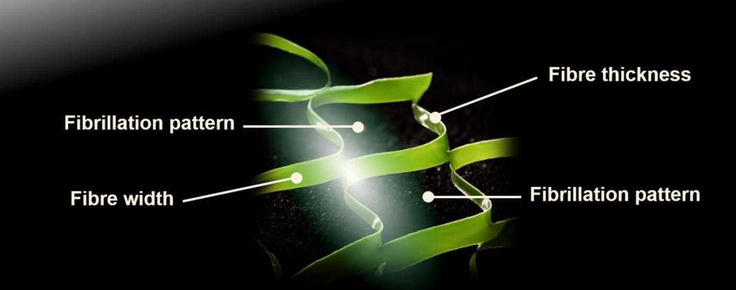
Unlike monofilament fibre, fibrillated yarn is produced as a wider tape before being semi split (fibrillation) into connected fibres. It has the advantage of being very durable, great at holding infill material in place, but not as good at staying upright. This means that it will flatten down far quicker and can thereby change the characteristics of the surface, which is not ideal for top level football. Its single colour also means it can be less attractive to look at.
